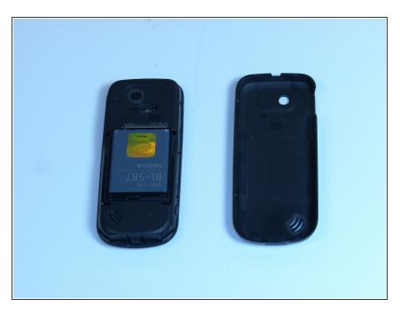
Remove the back cover to expose the battery.
