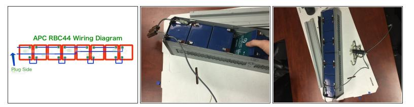
Use the wiring diagram made in step three to fill the cartridge with your brand new replacement batteries.
