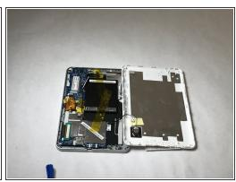
Open the back cover by prying the casing off with an opening tool.
