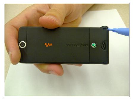
Place the plastic opening tool in the bottom corner of the phone in the crevice between the flap to remove the cover.
