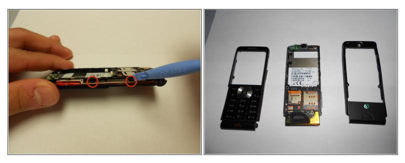
Using an opening tool and a gentle outward motion, separate the front plate from the inner phone workings.
