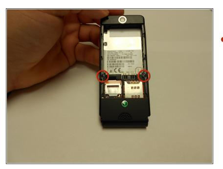
Using a mini Phillips screwdriver, remove two screws by turning them counterclockwise.
