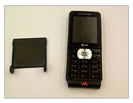
• Remove the cover with a slight twisting motion.
