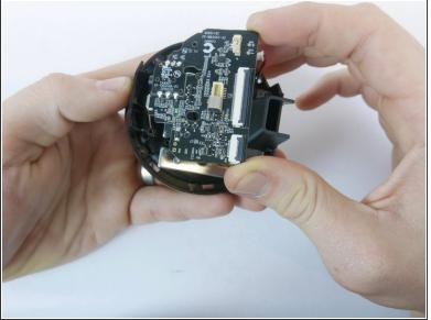
• Pull the board away from the bottom casing by lifting the end closest to the chimney up.
