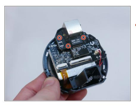
Use your Phillips #0 screwdriver to remove the three 5mm screws.
