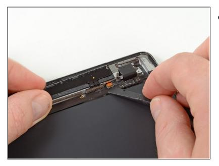
• Use the flat end of the spudger to pry up the antenna connector cable out of its socket on the headphone jack assembly board.
