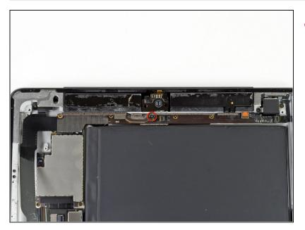
Remove the single 2.6 mm Phillips #0 screw securing the camera cable to the headphone jack assembly.
