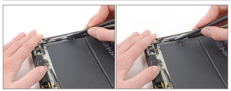
• Slide a spudger underneath the power & volume cables, releasing the adhesive.
