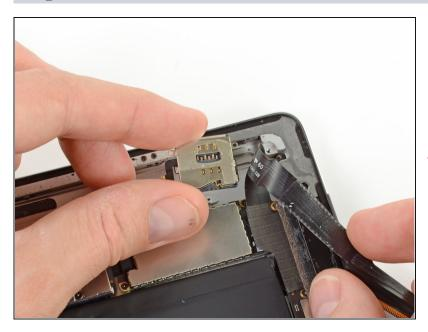
Holding the headphone jack assembly cable out of the way, remove the SIM board from the iPad.
