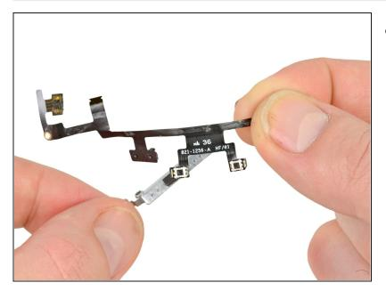
• Lift and remove the power & volume button ribbon cable.
