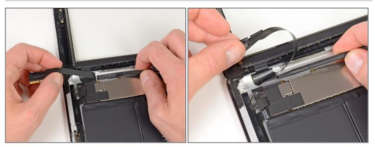
• Peel back the touchscreen ribbon cable and use the flat end of a spudger to release the adhesive securing the cable to the rear aluminum case.
