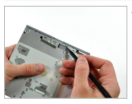
If necessary, use the tip of a spudger to release the two plastic bezel tabs from their slots on the bottom of the optical drive.
