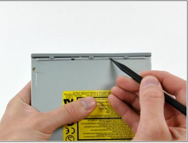
Use the tip of a spudger to push the two plastic bezel tabs away from their retaining slots on the top of the optical drive.
