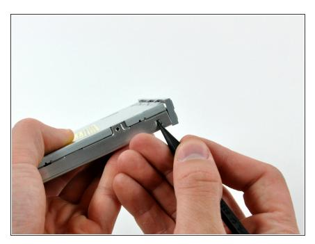
Use the tip of a spudger to depress and release the bezel retaining tab on the side of the optical drive.
