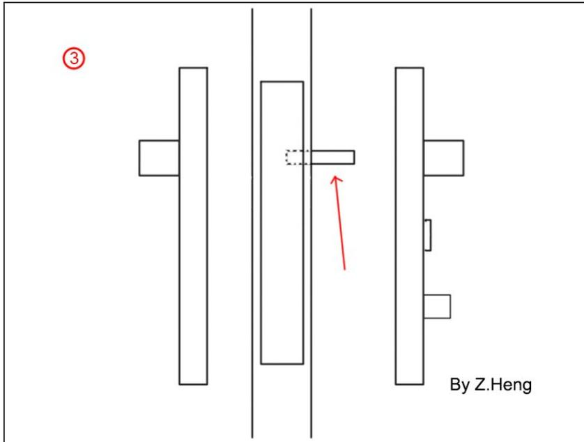
**⚠** Pay attention to the installation direction of this square shaft. Do not knock it off when removing the handle.
