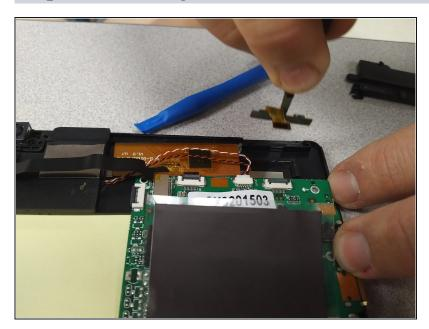
Using <u>tweezers</u> genitally pull up on the volume button board to remove.
