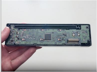
Use a spudger or prying tool to open the back of the face plate. Pry the back at multiple points around the edge of the face plate. This will take some patience. Applying too much force risks breaking the plastic.
