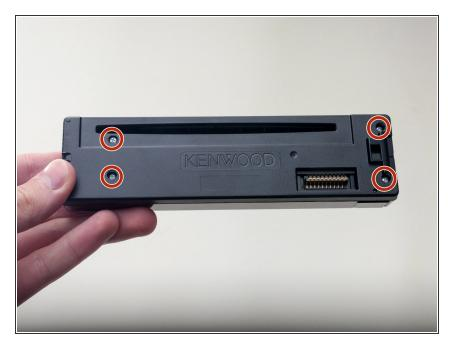
Remove the four 7.5mm Phillips #0 screws on the back of the faceplate.
