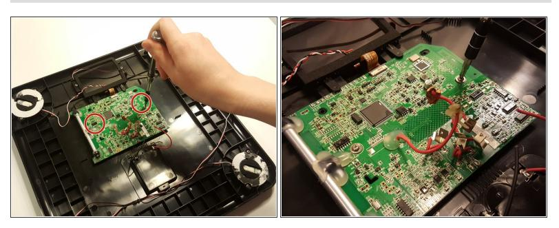
Using the Phillips-head screwdriver, unscrew the two screws that are securing the motherboard in place
