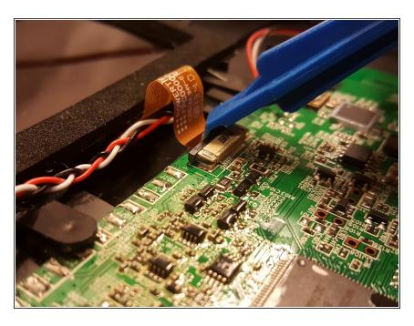
Using a plastic spudger, disconnect the LCD display's ribbon cable from the motherboard.
