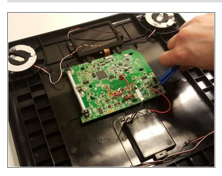
Once the two screws and the ribbon cable are detached, remove the motherboard.
