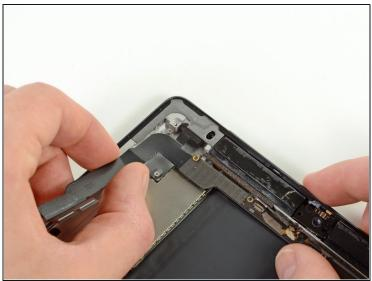
Holding onto the ribbon cable of the headphone jack assembly, carefully pull the assembly parallel to the iPad, toward the bottom of the device.
