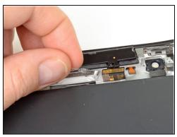
• Use the tip of the iSesamo or the edge of a plastic opening tool to remove the metal EMI tape covering the antenna cable.
