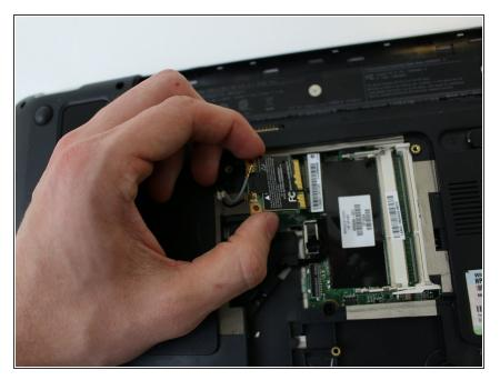
Gently lift the card upward and pull it out.
