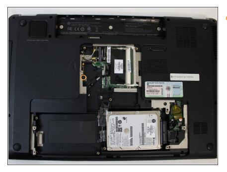
Remove the single screw underneath the black cable.
