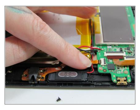
Move the wires out of the way and slowly pull the ribbon out of the circuit dock.
