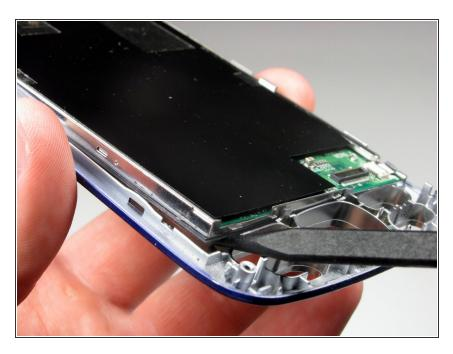
Use the spudger to unclip the screen in the lower left corner and gently pry it from its clips.
