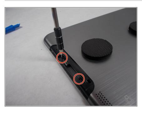
Use a Phillips #00 Screwdriver to unscrew the two 1.2mm screws within the compartment. This allows the device to be opened.
