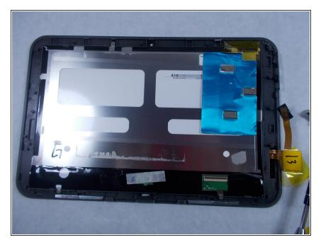
There are three silver tabs around the internal components that connect it to the frame with screws.
