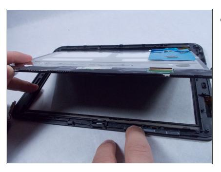
Carefully lift the internal components from the screen and place them into a replacement screen.
