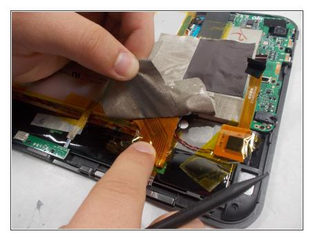
Remove the tape that is holding the battery in place.
