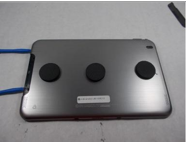
Insert opening tools to partially pry open the cover.
