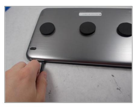
With the cover being partially held open, slide a spudger around the seam to pry off the cover.
