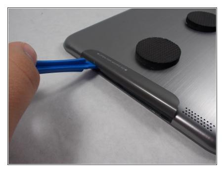
Use an opening tool to pry off the lid of the memory card compartment.
