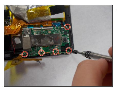
Unscrew the five 1.2mm screws that connect the circuit board to the device.
