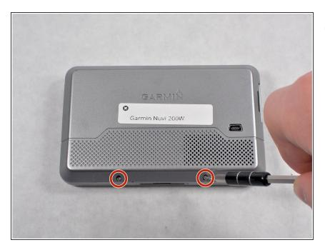
Remove the two 4mm T5 Torx screws.
