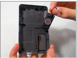
• Using the plastic opening tool, carefully apply pressure to lift the speaker up from the back cover.
