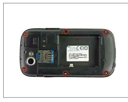
Remove the six Phillips screws securing the rear inner frame to the inner case.
