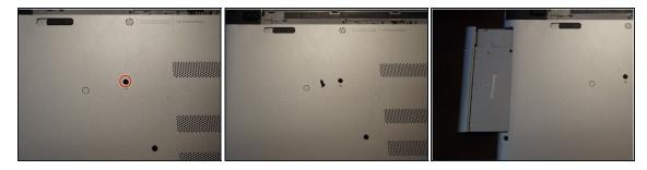
• Remove the screw that holds the optical drive in. To do this, use a **Phillips #0** screwdriver. Slide the optical drive out once this screw is removed.
