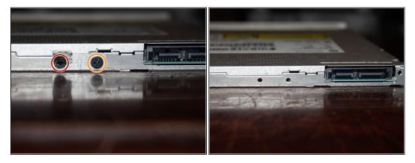
• Remove the screws holding the optical drive bracket onto the drive. To do this, use a *Phillips #0* screwdriver.
