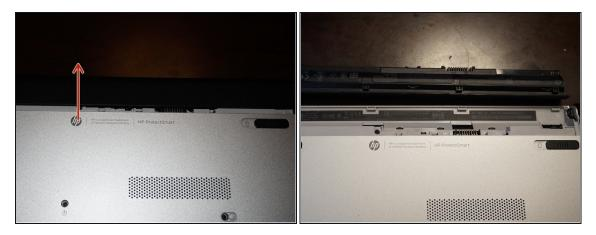
• Remove the battery. Pull the battery forward and remove it from the laptop.
