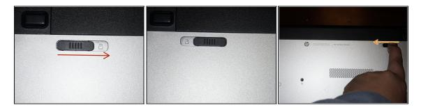
• Once the computer is off, remove the battery. Switch the locking tab to the unlocked position.
