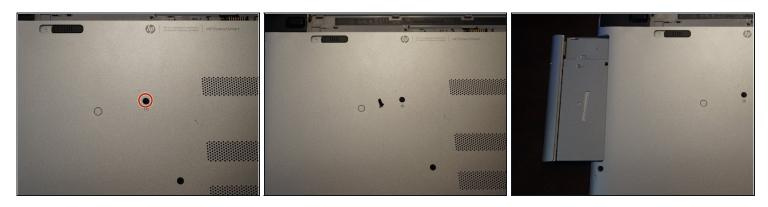
• Remove the screw that holds the optical drive in. To do this, use a **Phillips #0** screwdriver. Slide the optical drive out once the screw is removed.
