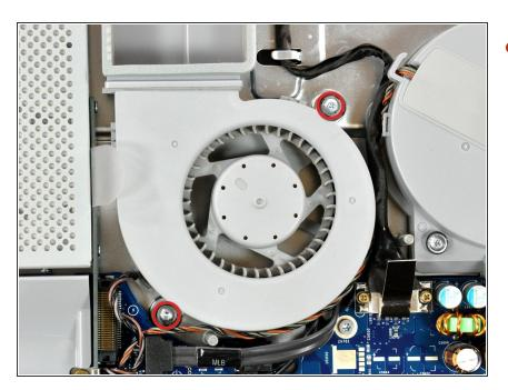
Remove the two 9.7 mm shouldered T8 Torx screws from the left fan.
