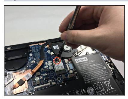
Use a #00 Phillips screwdriver to remove the 3mm screw in the center at the top of the card.
