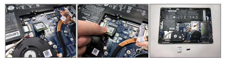
• The WiFi Card should be unbound from the surface. Carefully remove the card from the laptop by puling away from the socket.
