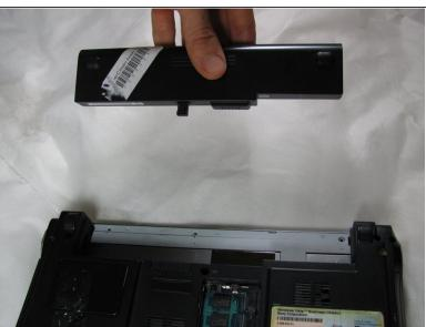
While holding the release slide with one hand, use your opposite hand to pull the battery from its slot by gently shaking the battery left and right to help slide it out.
