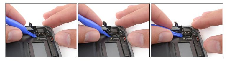
• Slide a plastic opening tool under the rear facing camera and pry upward to free it from the adhesive securing it to the rear case.
