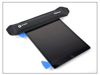
Heat an iOpener and apply it to the top edge of the device for two minutes.
