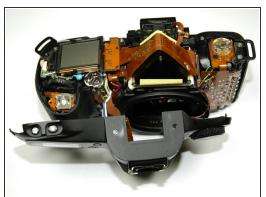
Remove the top panel by lifting it from the back, pushing it forward over the camera and letting it rotate down in front of the camera.
