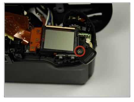
Unscrew the 6.8 Phillips screw that holds the strap anchor by the LCD.
