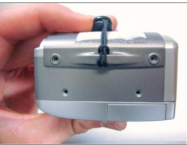
Remove the four 4.7 mm screws on the opposite side of the camera.
