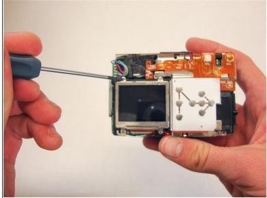
Using a Phillips #00 remove the four 4.40 mm screws that secure the LCD screen to the frame.
