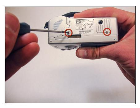
Use a Phillips #00 screwdriver to remove the two 4.7 mm screws in the bottom of the plastic casing.
