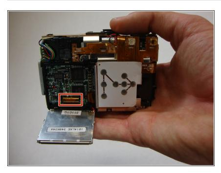
Allow the LCD screen to flip down.
