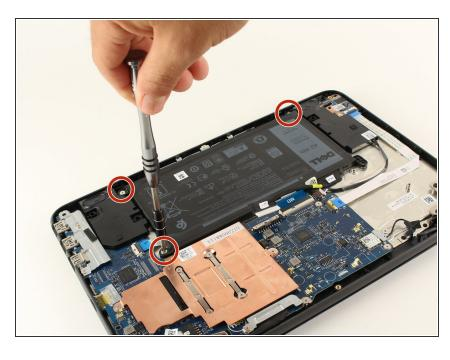
Using a Phillips #0 screwdriver, remove each of the three 3mm screws from the battery.
