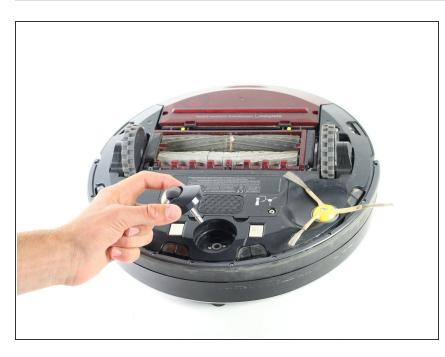
• Grip the caster wheel and pull it firmly out of its socket.
