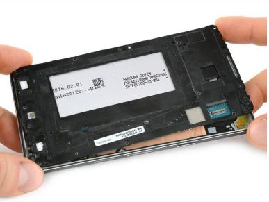
Push the top part towards the opened left side to rotate the midframe out.
