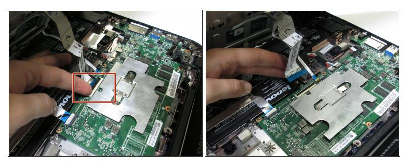
Disconnect the keyboard ribbon cable by lifting the ZIF connector lock with a plastic opening tool or fingernail and gently pulling the ribbon cable straight out of its socket.
