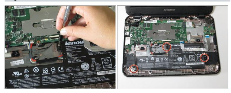
• Use a Phillips screwdriver to remove the three 3mm screws located along the edge of the battery.
