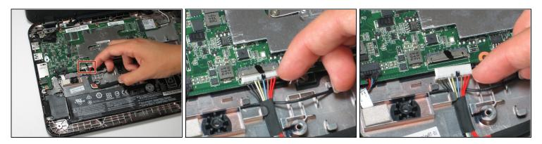
• Disconnect the white charging cable connectors by pulling straight down on the connector.
