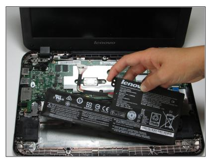
Remove the battery by pulling back and up.
