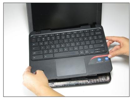
Remove the keyboard and trackpad panel away from the device.
