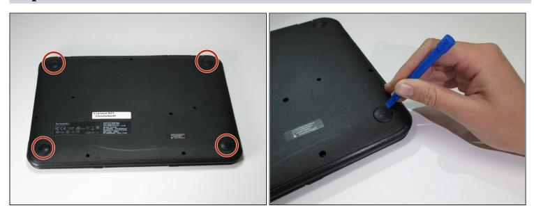
• Use a plastic opening tool to pry off the four rubber pegs from the bottom housing.
