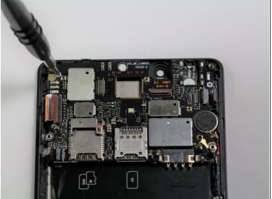
Remove the two 2.9mm Philips #00 screws.
