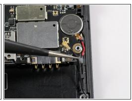
Locate the antenna cable on the bottom right of the motherboard and use tweezers to lift the cable off of the motherboard.
