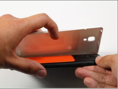
Run the plastic opening tool along the seam on the side of the phone to remove the rear casing.
