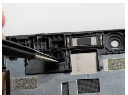
Use tweezers to pull out the rubber proximity sensor from the top left of the frame
