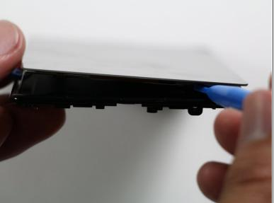
Run the plastic opening tool around the seam between the screen and the frame until an opening can be seen.
