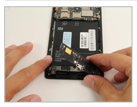
Lift the charging port up to remove it from the frame.
