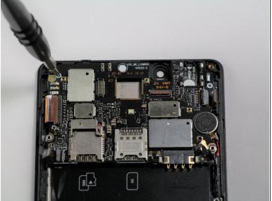
Remove the two 2.9mm Philips #00 screws.
