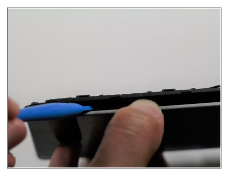
Slightly flex the frame to insert a plastic prying tool between the screen and the frame.
