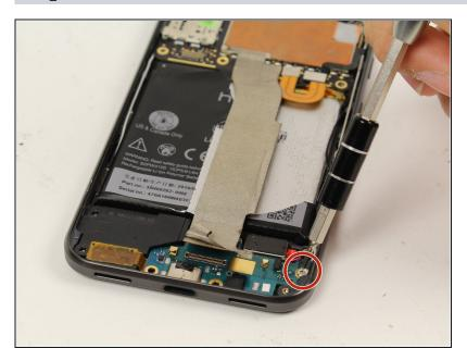
Remove the silver 2.5 mm T5 screw holding the daughterboard in place.
