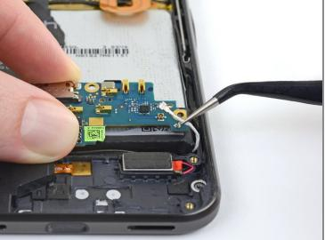
• Use tweezers to carefully pull each coax cable out of its retaining clip.
