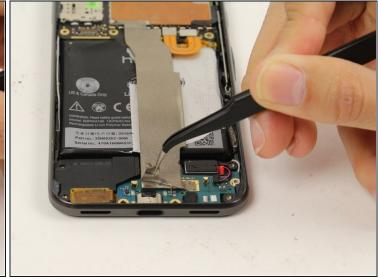
• Use <u>tweezers</u> to lift up the silver strip at the top of the daughterboard, and peel it back to expose the connector underneath.
