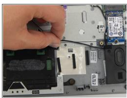
Pull the black wire out from under the the black center clips and up from the gray outer clips with a spudger.
