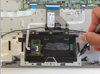
Remove the four 2.8 mm screws with a Phillips #00 screwdriver.
