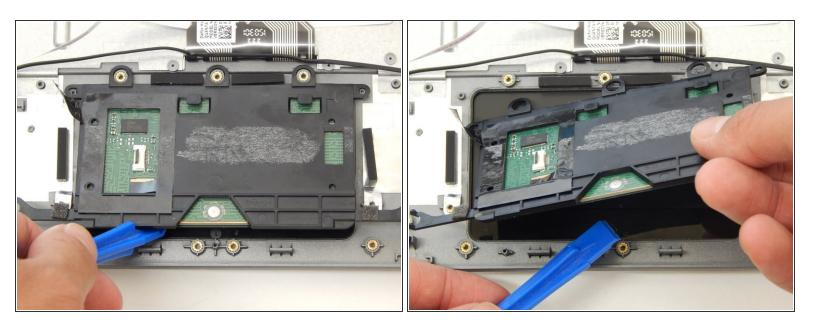
Lift off the black plastic cover with the plastic opening tool.
