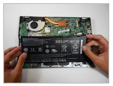
Lift the battery from the frame.
