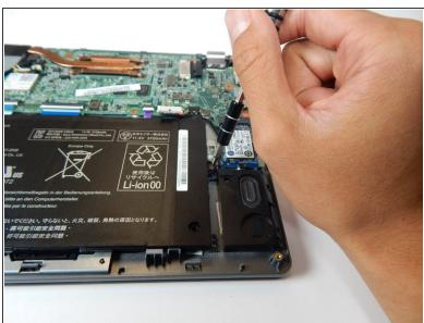
Remove the two 3.7 mm screws with a Phillips #0 screwdriver.
