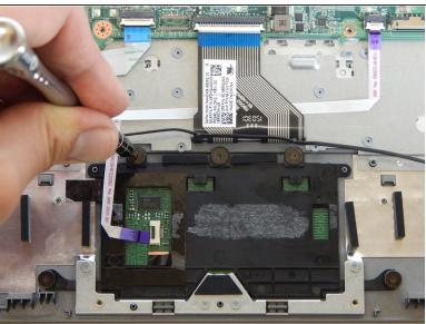
Remove the five 2.5 mm screws with a Phillips #0 screwdriver.
