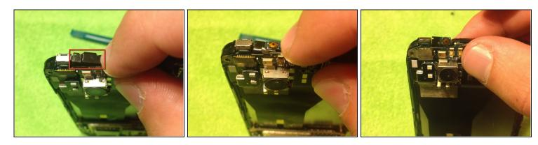
• Remove the same black plastic from the top power button. Be careful to only remove the plastic as there is a flex cable under.
