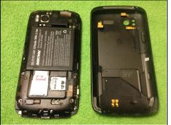
• DO NOT pry loose as shown in this picture. The button in the middle that is pictured can be pressed in, releasing the back housing which can then be easily lifted free.
