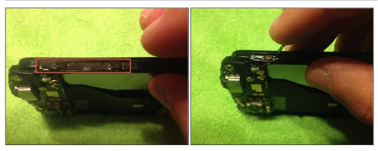
• Remove the black plastic covering the volume buttons on the side.
