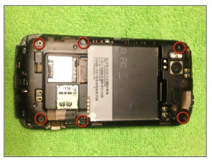
Using a Torx screwdriver, remove the 6 screws show in the photo.
