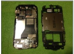
• Using a plastic pry tool, at the top, the right and left sides and the bottom, carefully insert and pry to pop loose the plastic frame from the LCD/Touchscreen Housing.
