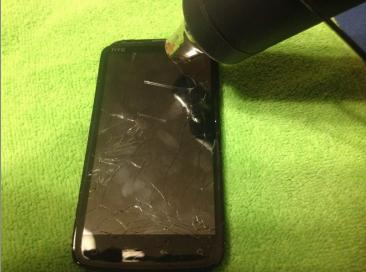
Using a heat gun, carefully heat the glass all around the screen. Be careful not to overheat as this can cause damage to the LCD.
