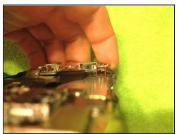
• With the power button flex up you can now carefully pull up the motherboard.
