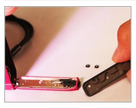
Using your fingers, remove the battery/memory card door seal.
