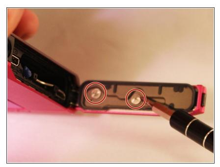
Using a Phillips #00 screwdriver, remove the two 2mm screws on the battery/memory card cover seal.
