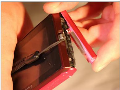
Pull the edge-casing off of the camera.
