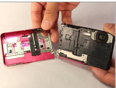
Remove the front casing of the device.
