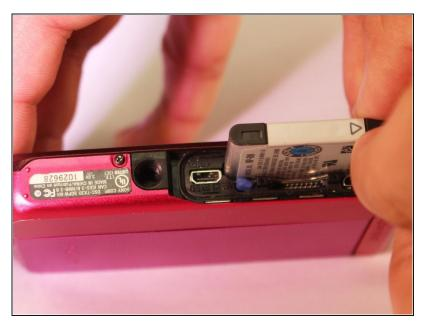
• Remove the battery from the device.
