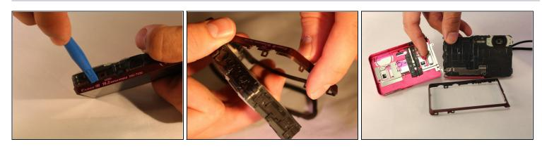
Using the plastic opening tool, remove the back casing of the device.
