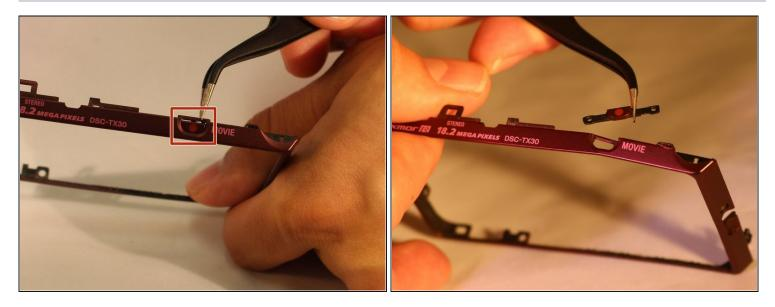
• Using the <u>tweezers</u>, remove the movie button from the back casing of the device.
