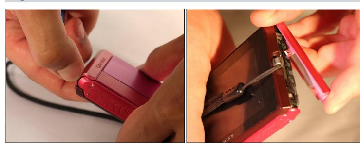
• Pull the edge-casing off of the camera.
