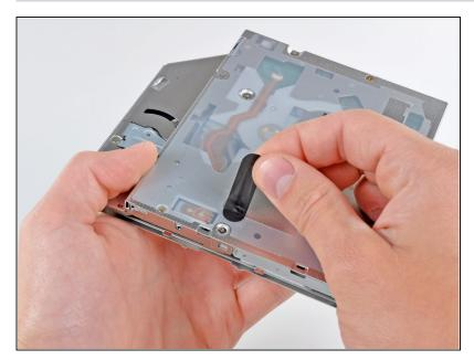
Peel off the strip of black tape covering the optical drive thermal sensor.
