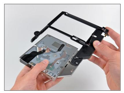
Remove the optical drive bracket from the optical drive, minding any cables that may get caught.
