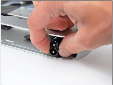
• Rotate the AC-In connector 90 degrees counter-clockwise.
