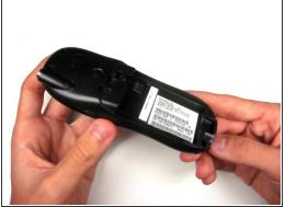
Remove the battery by pushing the bottom end towards the top, then lifting up.
