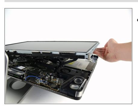
Lift and remove the display panel from the device.
