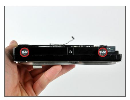
Remove the two T8 Torx screws and their attached rubber grommets from the hard drive.
