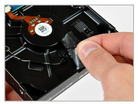
Peel off the piece of foam tape covering the hard drive thermal sensor.
