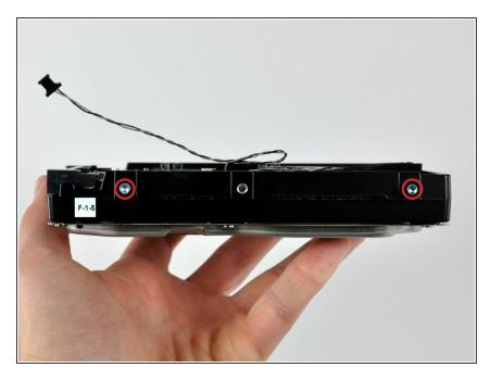
Remove the two T8 Torx pins from the side of the hard drive nearest the power and data connectors.
