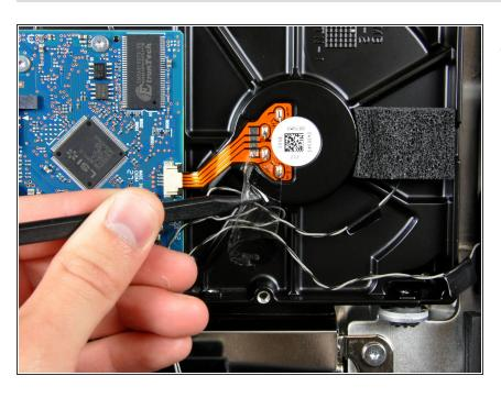
If present, remove the small piece of tape covering the hard drive and optical drive temperature sensor cables.
