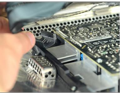
While still holding the display panel up, use two fingers to firmly push down on the power supply cable connector from its socket.
