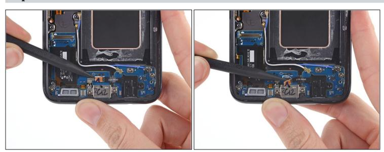
• Use the point of a spudger to disconnect the headphone jack connector.
