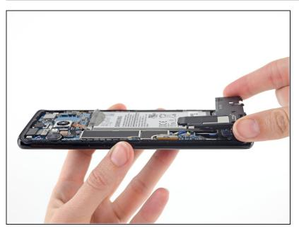
• Remove the loudspeaker assembly.
