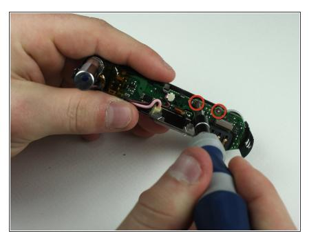
Unscrew the small screws beneath the top cover(#00P, 1.7mm).
