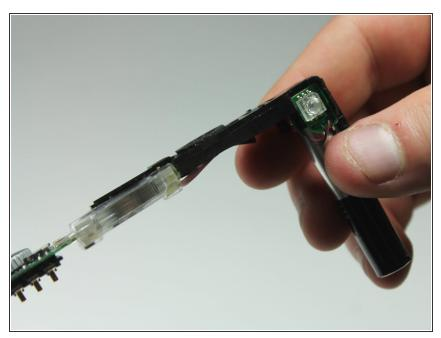
The flash assembly is hardwired into the top circuit board.
