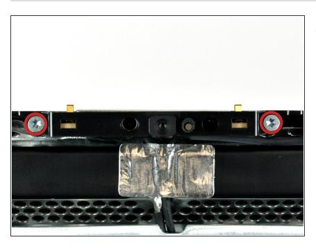
Remove the two T8 Torx screws securing the camera board to the rear case.
