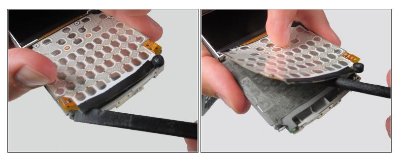
• Insert the flat edge of the spudger to the space under the keypad and slide it along the bottom to lift the keypad out of its place. The keypad should be stuck to the surface very tightly.
