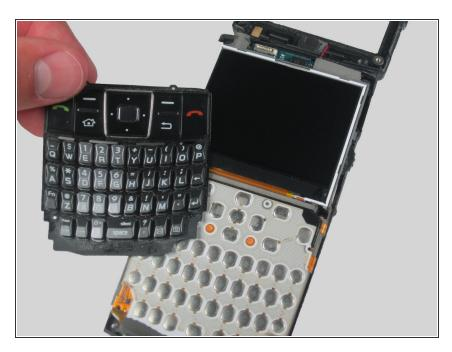
• Remove the keypad and place it to the side.
