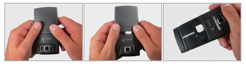
• To remove the back casing, firmly press down and push towards the bottom of the phone.
