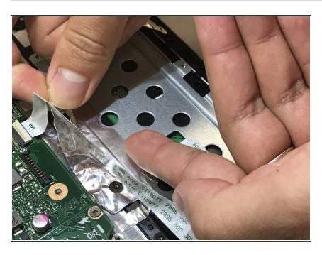
Remove all of the metallic tape holding the metal bracket to the components surrounding it.
