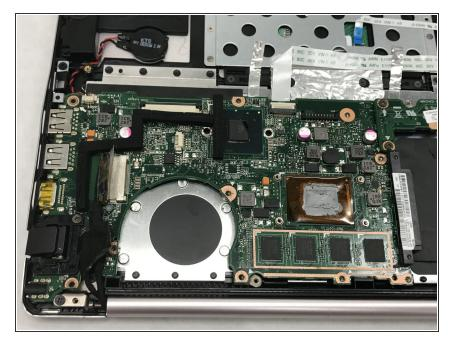
Locate the motherboard under the cooling fan.
