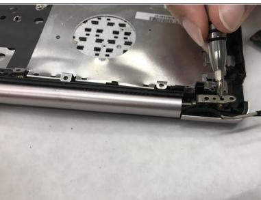
Next, unscrew the two 4.9mm hinge screws with a Phillips #00 screwdriver.
