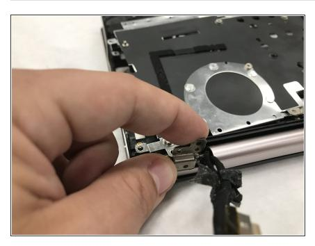
Pull the display hinges back in order to remove the metal keyboard panel.
