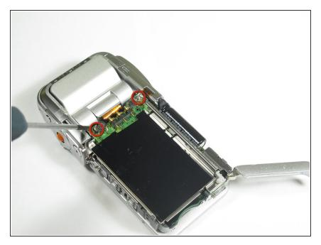
• Unscrew the two screws (5.18mm Philips) indicated by the picture.
