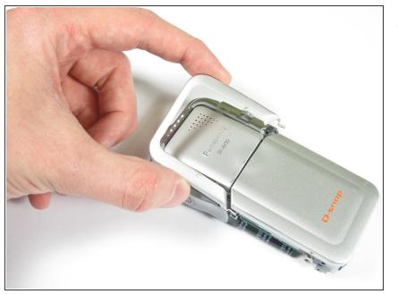
Remove the top piece of the casing from the camera, as shown in the picture.
