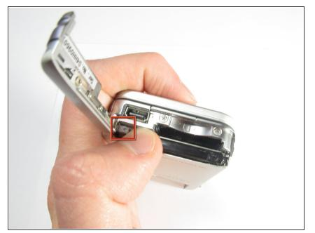
• Push the small gray plastic tab away from the battery in order to release the battery.
