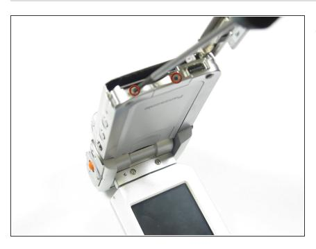
Remove the two screws (2.2mm Philips) indicated.
