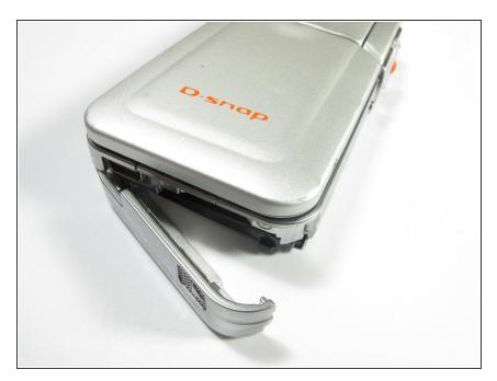
• Pull/lift open the battery cover in the direction directly away from the camera.
