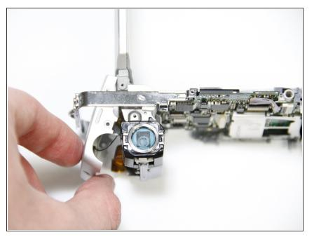
Carefully remove the other side of the lens casing by pulling it away from the lens, and make sure to keep attached to the wire it is connected to.
