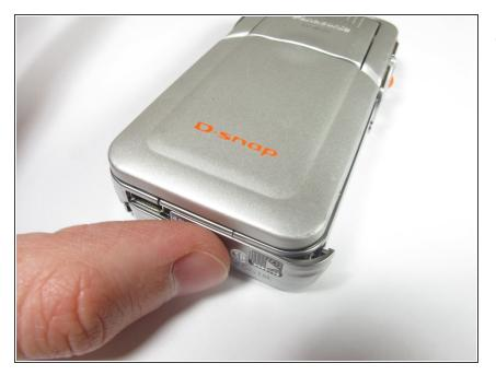
• Slide the bottom panel in the direction of the arrow on the panel.
