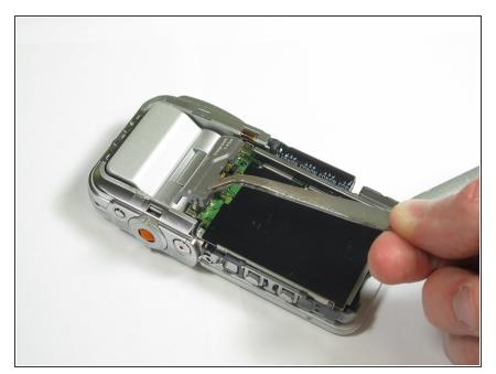
Remove the small cover from near the top of the motherboard, using tweezers or forceps, as in the picture.
