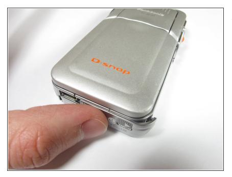
• Slide the bottom panel in the direction of the arrow on the panel.
