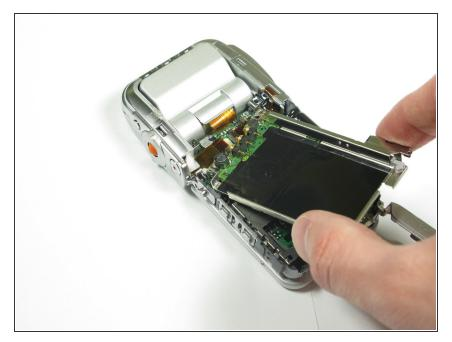
• Carefully remove the motherboard from the camera by grasping the sides and pulling upwards and then outwards.
