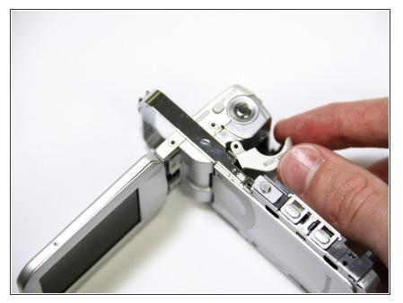
Carefully remove the bottom of the lens casing by pulling downwards away from the lens.
