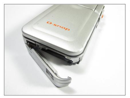
Pull/lift open the battery cover in the direction directly away from the camera.
