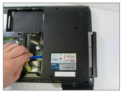
Use the plastic opening tool to push the drive out from the back.
