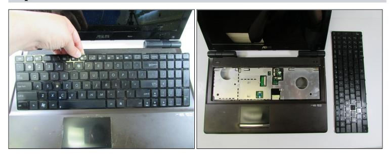
• Last, remove the keyboard completely from the computer.
