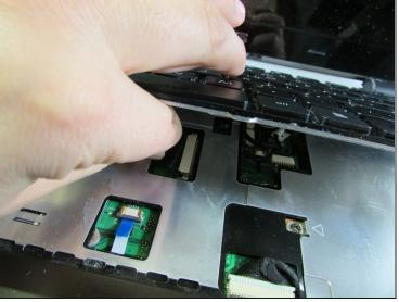
• Once the keyboard is free, lift it up slightly and release the cable connection underneath.
