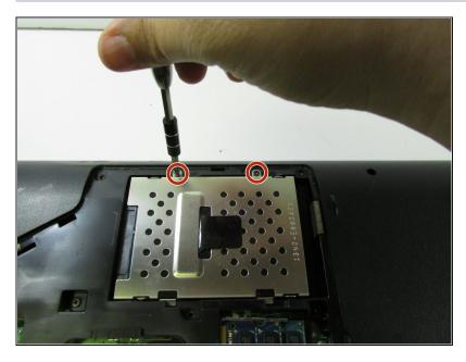
• Remove the two screws using a Phillips #1 screwdriver.
