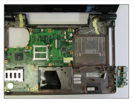
• Lift up and remove the port panel.
