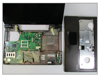
• Lift up and remove the upper case.
