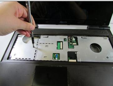
• Remove the two screws from the metal frame.
